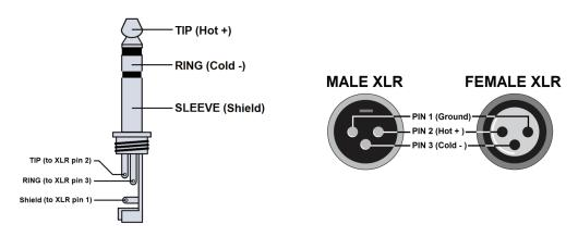
Telos recommends connecting your Hx1 / Hx2 to professional-grade audio equipment with balanced audio connections. If your Hx1 / Hx2 must connect to semi-pro "unbalanced" audio inputs or outputs, we recommend using a two-way, external balanced / unbalanced line level converter. Common models include the "Matchbox", "ProMatch", and "CleanBox Pro", as well as other model names.
